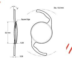
One-piece aspherical biconvex hydrophilic acrylic lens with soft-aberration system
